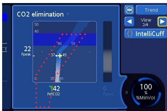
The CO 2 elimination map shows the patient's PetCO 2 value and the defined target zone (light-blue boomerang-shaped window).
